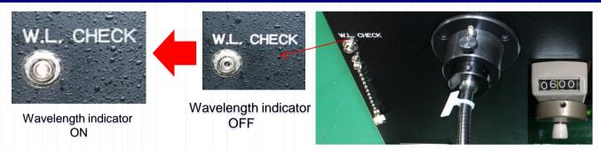
When selecting the wavelength at 600nm for an example, the wavelength indicator lights if there is any problem on the system.
