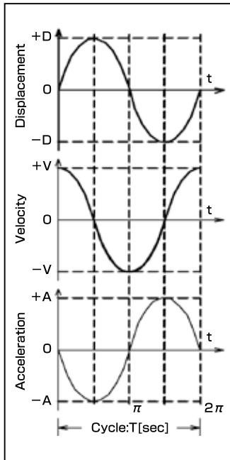
Relations between the frequency of sine wave vibrations and displacement, velocity and acceleration.
